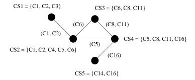
The lower bound can be computed by a polynomial algorithm. Indeed, the problem consists of finding an EDGE COVER of the graph. In the EDGE COVER problem the goal is to find the minimum number of edges required to cover all the vertices. In [12,6] the EDGE COVER problem is mentioned to be solvable by matching algorithms. Let us go further in details. We call d(x) the number of edges incident to a vertex x in a graph G (the degree of x).
